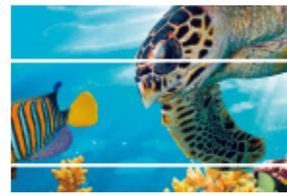
Gap/White streaks (Excessive feeding amount)
