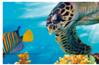
Overlap/Black streaks (Insufficient feeding amount)
