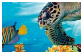
Overlap/Black streaks (Insufficient feeding amount)
