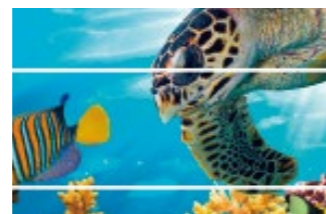
Gap/White streaks (Excessive feeding amount)
